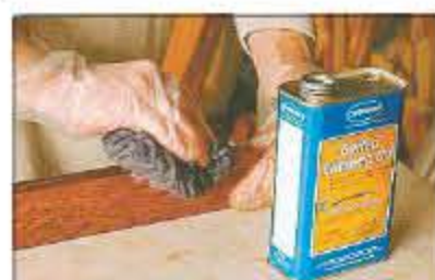
Dinger rubs boiled linseed oil on a piece of reclaimed oak board for a small table.
